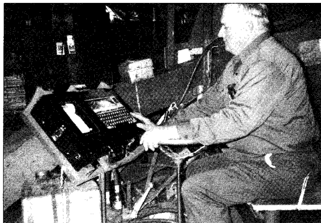
Researchers at Agripro, a major seed company, in conjunction with the Jacobsen Holz Corporation, use a Model 102 housed in a briefcase and attached to a mechanical harvester to collect needed data.
