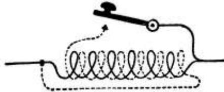
Fig. 129. DIFFERENTIAL WINDING WORKING OF ELECTRO-MAGNETIC APPARATUS.
