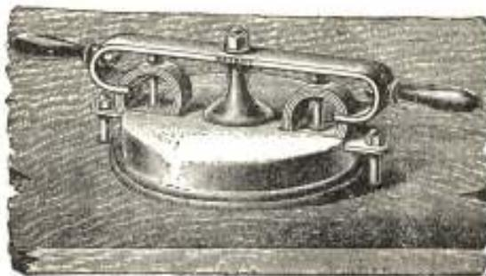
Fig. 298. SWITCH WITH RING CONTACTS.
