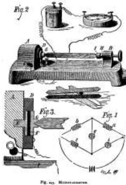
Fig. 243. MICROTASIMETER.
