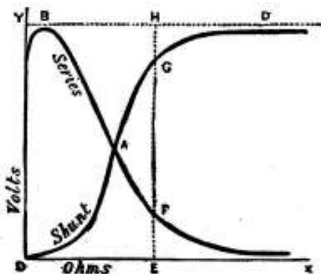
Fig. 350. CHARACTERISTIC CURVES OF SHUNT AND SERIES WINDING.
