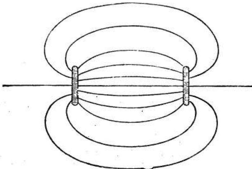
Fig. 162. ELECTROSTATIC LINES OF FORCE BETWEEN DISTANT SURFACES.
