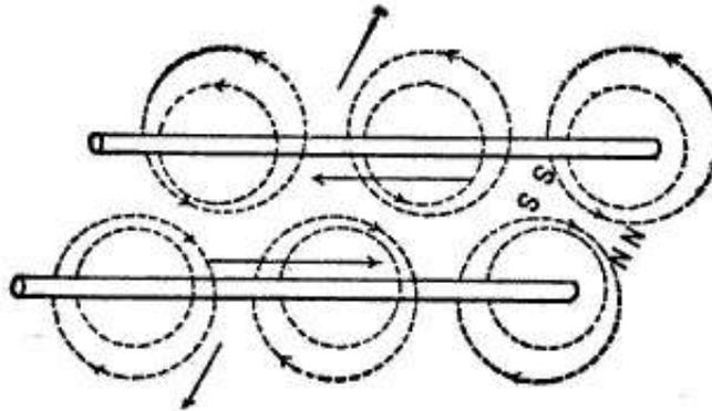
**Fig. 201. REPULSION OF CONDUCTORS CARRYING OPPOSITE CURRENTS.**
