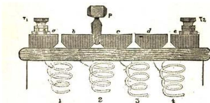
Fig. 104. RESISTANCE COILS AND CONNECTIONS, SHOWING PLUG.
