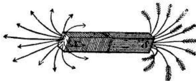
Fig. 223. MAGNETIC LINES OF FORCE, DIRECTION OF.
