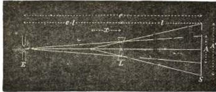
Fig. 260. DIAGRAM OF PRINCIPLE OF THE DISPERSION PHOTOMETER.
