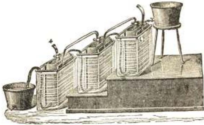
Fig. 40. CAMACHO'S BATTERY.
