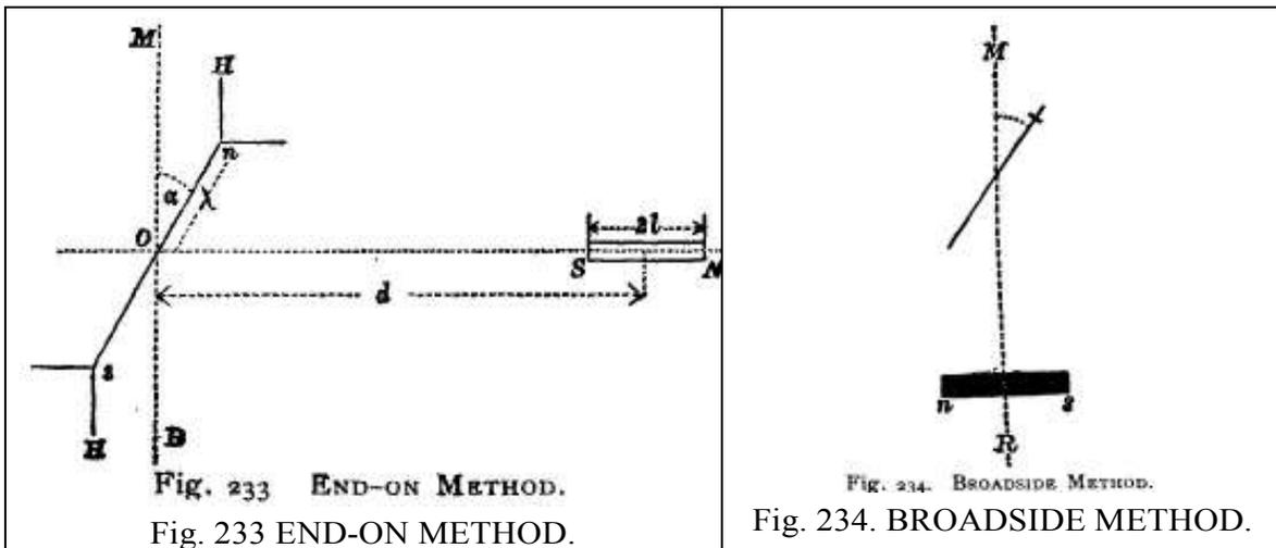
$M/H$  is determined by the End-on deflection method, or the Broadside deflection method. In both cases the deflection of a compass needle by the magnet in question is the basis of the work.
