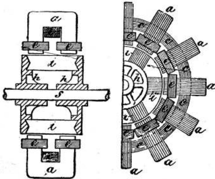
Fig. 202. INDUCTOR DYNAMO.
