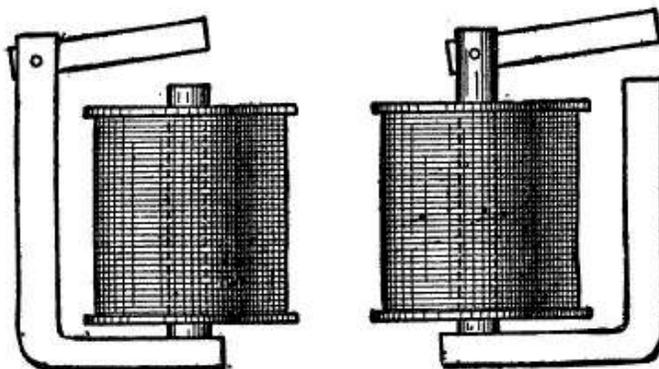
Fig. 26. HINGED ARMATURES OF CLUB-FOOT ELECTRO MAGNETS.
