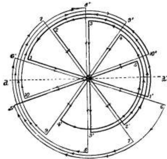
Fig. 25. PLAN OF WINDING PACINOTTI'S DISC ARMATURE.
