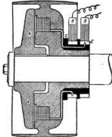
Fig. 94. ELECTRO-MAGNETIC CLUTCH.
