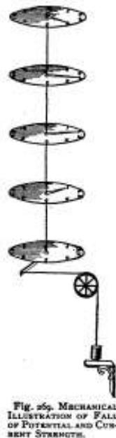
Fig. 269. MECHANICAL ILLUSTRATION OF FALL OF POTENTIAL AND CURRENT STRENGTH.
