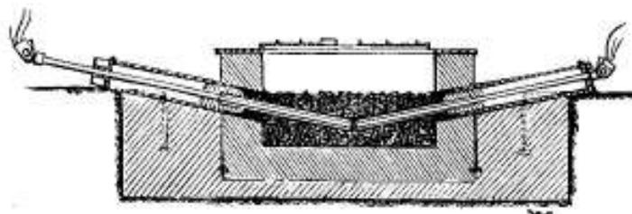
Fig. 175. CRUCIBLE, ELECTRIC.
