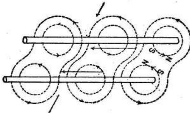
**Fig. 200. ATTRACTION OF CONDUCTORS CARRYING SIMILAR CURRENTS.**
