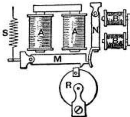
Fig. 151. INTERLOCKING ELECTRO-MAGNETS.
