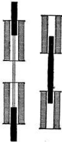
Fig. 97. DIFFERENTIAL COILS AND PLUNGERS.
