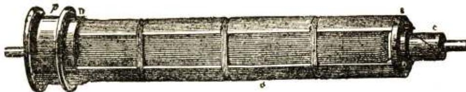
Fig. 32. SHUTTLE OR H ARMATURE.
