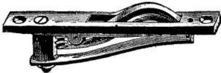
Fig. 9. BURGLAR ALARM SWITCH OR CIRCUIT BREAKER.
