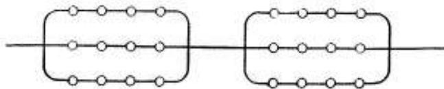
Fig. 302. SERIES-MULTIPLE CONNECTION.
