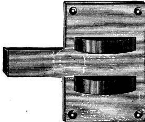
Fig. 8. BURGLAR ALARM SWITCH OR CIRCUIT BREAKER.
