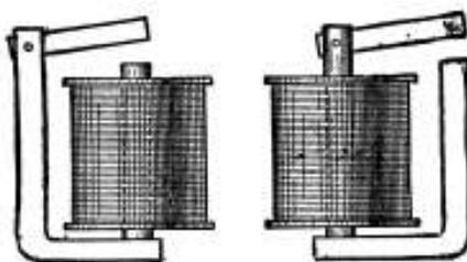
Fig. 148. CLUB-FOOT ELECTRO-MAGNETS WITH HINGED ARMATURES.
