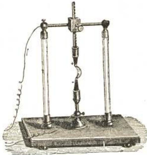
Fig. 19. EXPERIMENTAL APPARATUS FOR PRODUCING THE VOLTAIC ARC.
