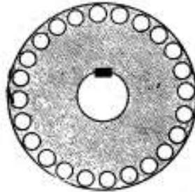
FIG. 114. PIERCED OR PERFORATED CORE-DISC.
