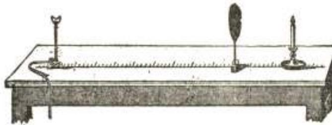
Fig. 259. BAR PHOTOMETER.
