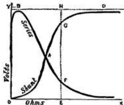
Fig. 137. CURVES OF SERIES AND SHUNT WINDINGS SUPERIMPOSED.
