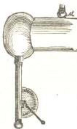
Fig. 157. HENLEY'S QUADRANT ELECTROSCOPE.
