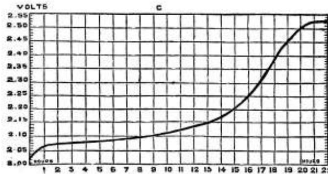
Fig. 121. CHARGING CURVE OF A SECONDARY BATTERY.
