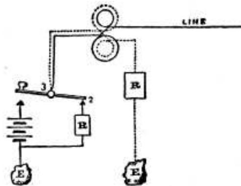
Fig. 316. DIFFERENTIAL DUPLEX TELEGRAPH CONNECTIONS.
