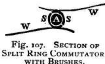
Fig. 107. SECTION OF SPLIT RING COMMUTATOR, WITH BRUSHES.
