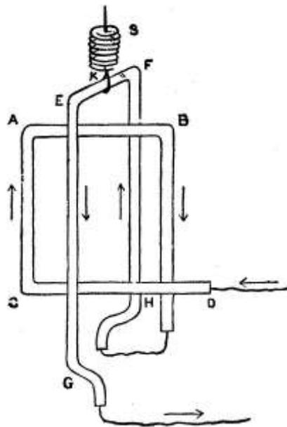
Fig. 143. DIAGRAM OF CONNECTIONS OF SIEMENS' ELECTRO-DYNAMOMETER.
