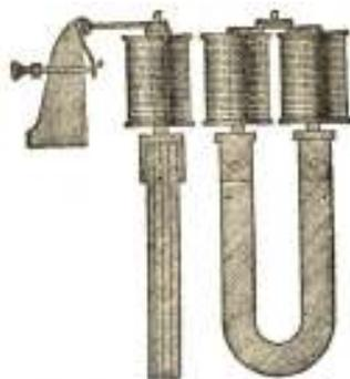
Fig. 317. ELECTRO-MAGNET OF HUGHES' PRINTING TELEGRAPH.
