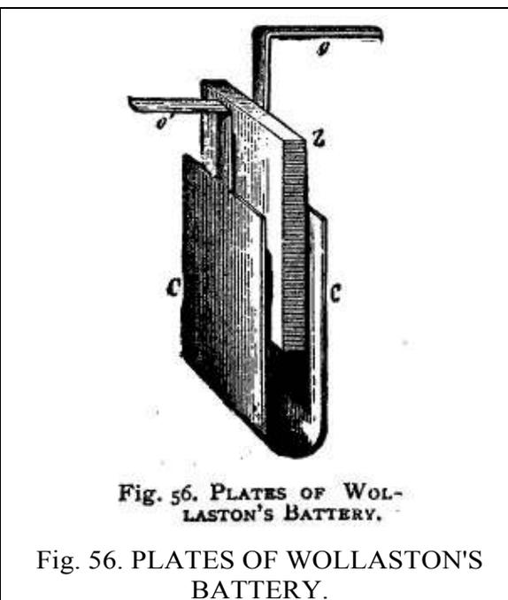
**Battery, Wollaston.** The original plunge battery is attributed to Wollaston. He also invented the battery known by his name, having the disposition shown in the cut, of zinc *Z*, surrounded by a thin sheet of copper *C*; *o*, *o'*, *o''*, are the terminals and *B*, *B*, the battery jars. Dilute sulphuric acid is used for exciting fluid.
