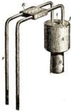
Fig. 292. STANDARD OHM COIL.
