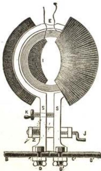
Fig. 102. INVERTED INDUCTION COIL FOR ELECTRIC WELDING.
