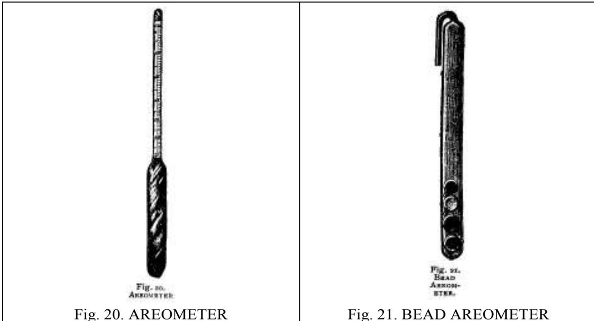
**Areometer, Bead.** A tube of glass containing beads of different specific gravities. It has apertures at top and bottom. When immersed in a liquid, the same fills it, and the specific gravity within certain limits, depending on the factors of the beads, is shown by the beads which float and those which sink. It is used for storage batteries and other purposes where acids and solutions have to be tested.
