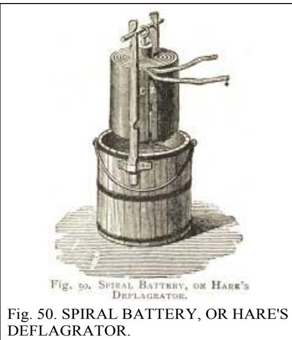
**Battery, Spiral.** A battery whose plates of thin zinc and copper are wound into a spiral so as to be very close, but not touching. Dilute sulphuric acid is the excitant. It is now practically obsolete.
