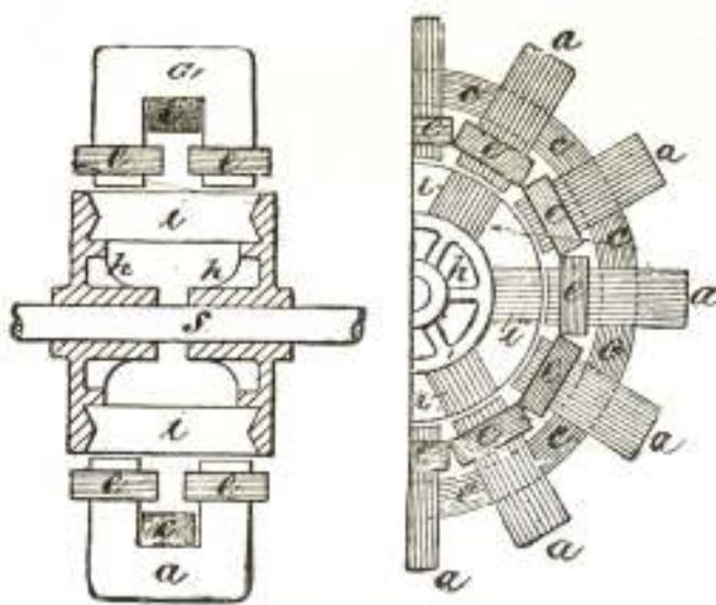
FIG. 139. INDUCTOR DYNAMO.
