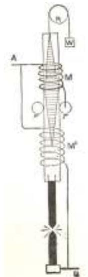
Fig. 211. DIAGRAM OF THE PILSEN DIFFERENTIAL ARC LAMP.
